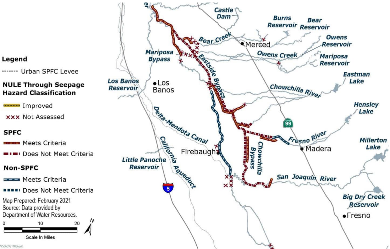
Figure 5-20. Non-Urban Levee Evaluation Project Through-seepage Hazard Classifications
