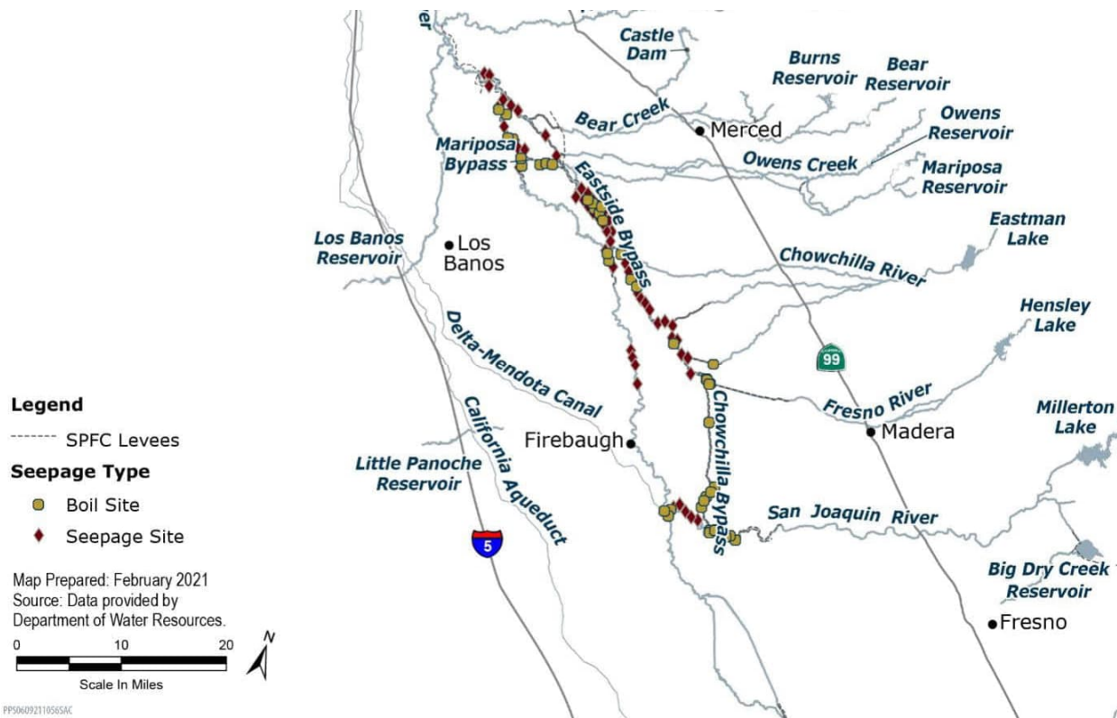
Figure 5-22. Historical Boil and Seepage Sites
